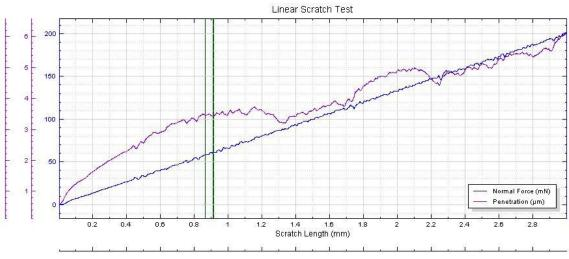
Figure 7 : Loading Curve – Plastic
