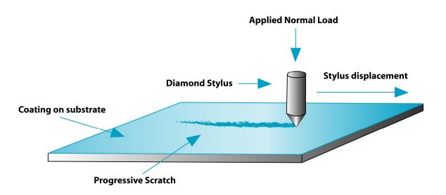
Figure 1 : Principle of scratch testing
