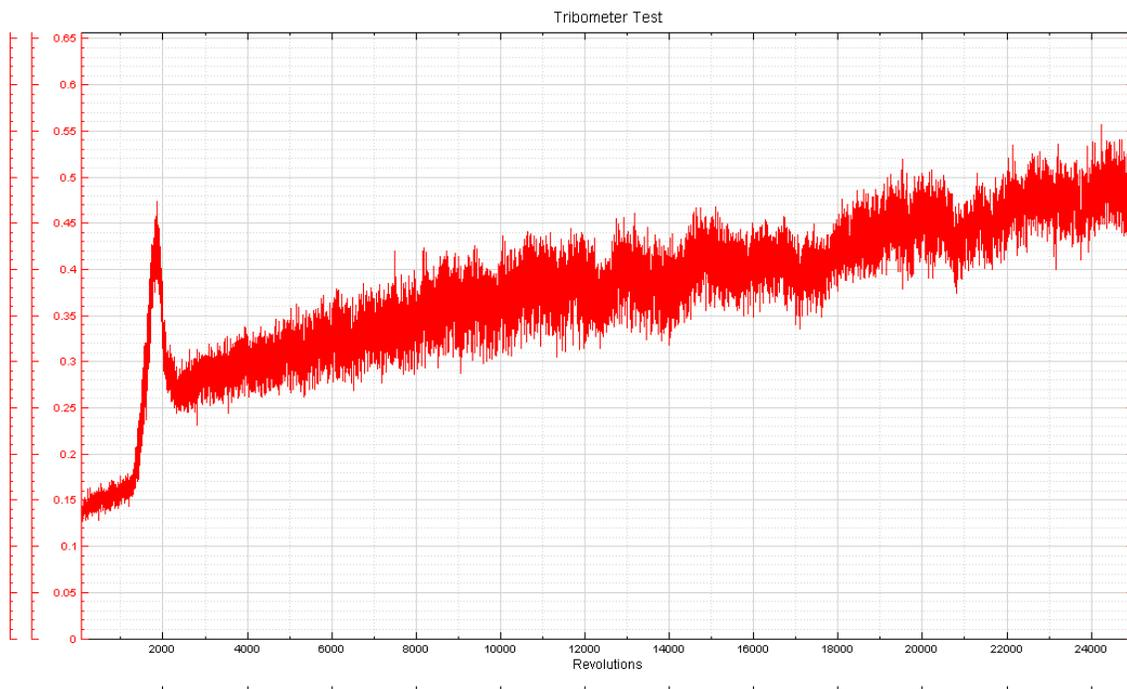
Figure 4: Graph of coefficient of friction – Sample X
