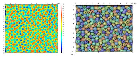
Mean Area: 0.394016mm<sup>2</sup> | Mean Volume: 0.000408109mm<sup>2</sup> Mean of Mean Diameters: 0.683262mm | Mean Form Factor: 0.638741 Mean Aspect Ratio: 1.67253 | Mean Roundness: 0.636164
