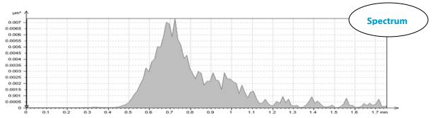
Power spectrum density is displayed here to show dominate wavelengths around 0.68mm and 0.74mm, with minor peaks up to 1.72mm.
