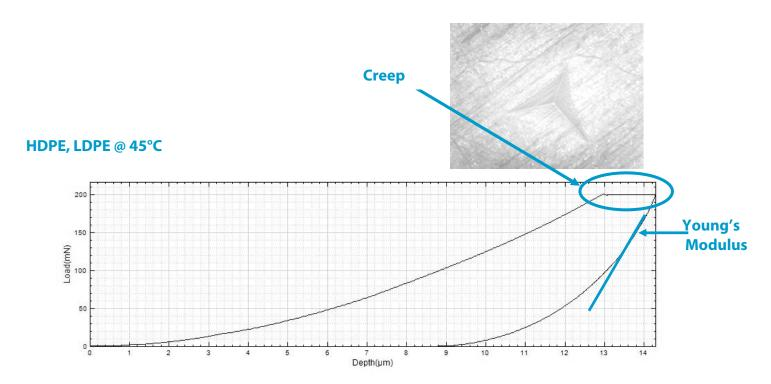
Here, the graphs at elevated temperature testing looked similar to that of the room temperature but with a difference in depth. Larger depths are achieved during heating of the polymer due to the softening material.
