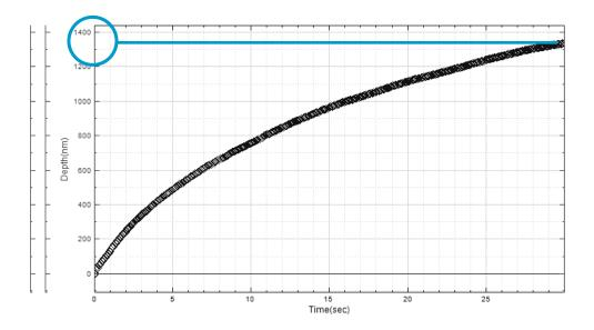
In this case, we can determine the displacement during a creep time of 30 seconds is 1.37microns. Again, because the polymer is at higher temp larger displacements are also observed during creep time.
